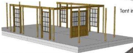
Wood legs with windows and doors installed
