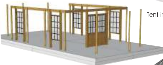
Wood legs with windows and doors installed
