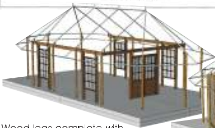
Wood legs complete with steel structure
