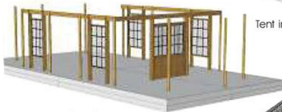
Wood legs with windows and doors installed
